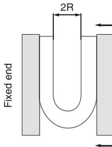
At a temperature of 20°C, bend the tubing into a U shape. Fix one end and gradually move the other end closer. Measure 2R at the point where the outside diameter's rate of change is 10%.
