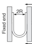
Bend the tube into U-form at a temperature of 20°C. Fix one end and close loop gradually. Measure 2R when the tube breaks or is crushed.
