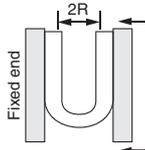
At a temperature of 20°C, bend the tubing into a U shape. Fix one end and gradually move the other end closer. Measure 2R at the point where the outside diameter's rate of change is 10%.
