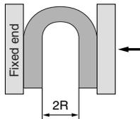
At a temperature of 20°C, bend the tubing into a U shape. Fix one end and gradually move the other end closer. Measure 2R at the point where the outside diameter's rate of change is 5%.
