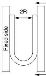
At a temperature of 20°C bend the tubing into a U shape. Then with one side fixed, gradually close the other side and measure 2R at the point where the tubing folds or flattens, etc.
